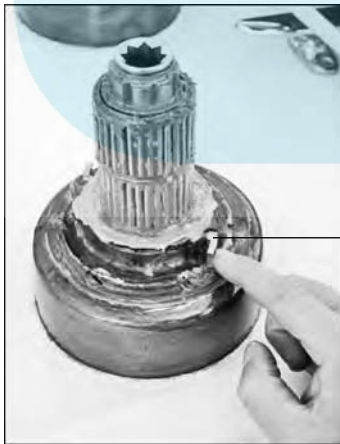
Figure 15-5: Checking the pawls and their springs inside a winch.
